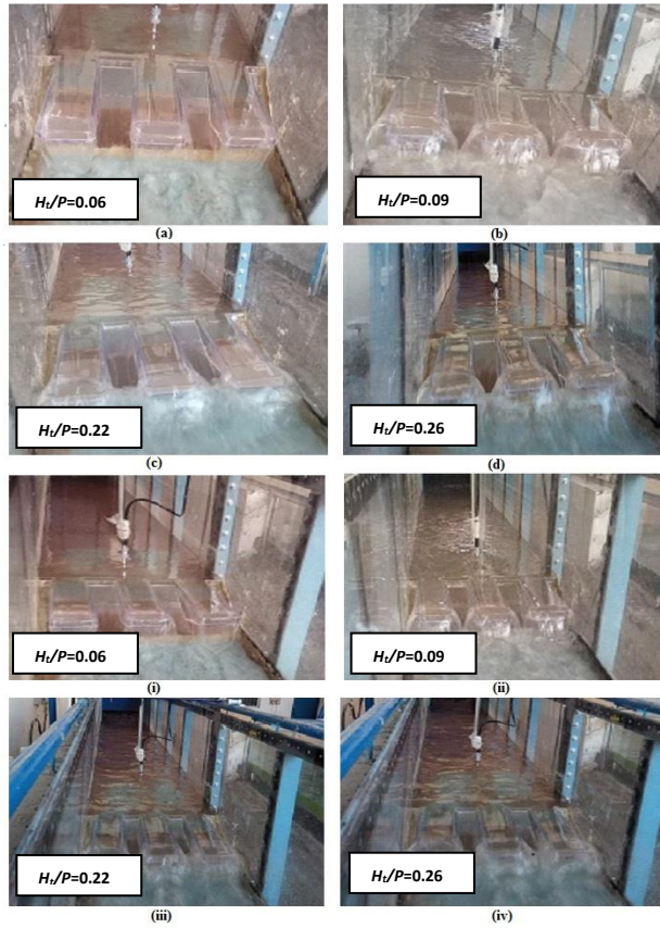
Figure: 6. Shows the surface tension effects to jet trajectory formation from (a) to (d) on Largest models and from (i) to (iv) on Smallest models.
