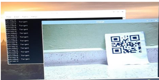
Fig.5 Decoding the input QR code and command to motor
