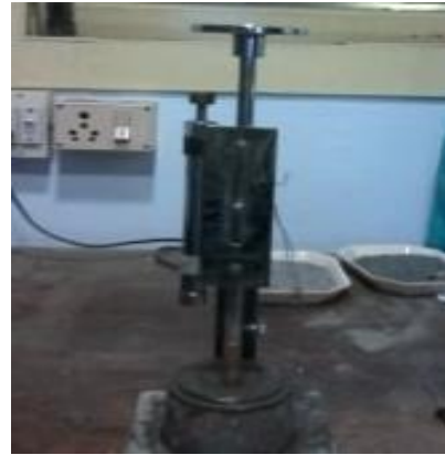
Figure 3.2 Setting Time Test for Cement
